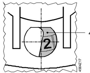
Display window with scale dial (4) and stroke
