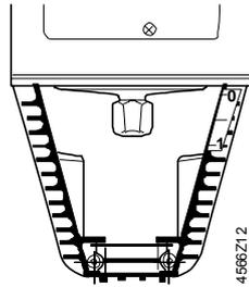
Cylinder with valve stem connector fully extended
