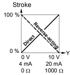
Note The mechanical spring-return function is not affected by the direction of operation selected.
