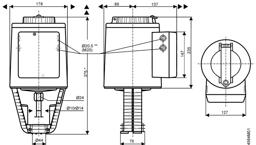
\*\* **SKC..U:** with knockouts for standard ½" conduit connectors (Ø 21.5 mm)
