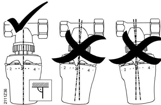
When mounting the actuator to the valve, ensure that valve and actuator form a right angle.
